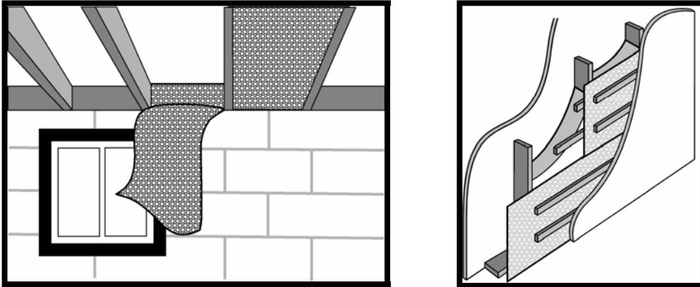
There are other beneficial considerations for using reflective insulation. Generally, these products have a very low water vapor and air permeance. When installed properly, with joints taped securely, reflective insulation materials are efficient vapor retarders and an effective barrier to air and radon gas.
