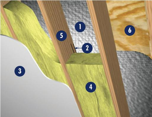
Northern Zone of the USA -With Reflectix® Below the Mass Insulation • R-7.0 Summer & R-1.0 Winter and a Vapor/ Moisture Barrier
